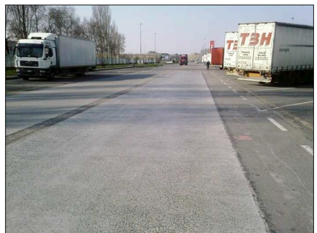
Figure 2: Test field on bitumen-cement photocatalytic paving, 2011
